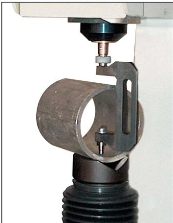
By applying C shape indeter Art. 604, difficult points as: insides of tubes and near to hollows can be reached.
