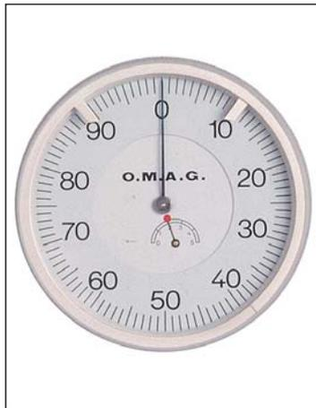
classic Rockwell's principle with direct Rockwell's hardness on a large dial.
